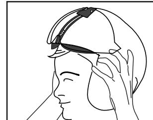
Helmet wearing is given by the low position of the inner visor (except for LH 150 given by outer visor)
